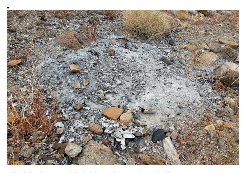
• This six foot diameter mound of melted aluminum in the burned area looked like concrete.
