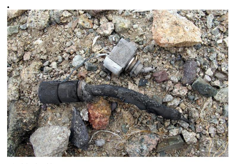
• A switch and coaxial connector.
